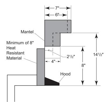
Figure 10 is an example of an unsafe mantel installation. This mantel projects 4" at 8" above the opening, exceeding the maximum acceptable distance of  $2^{1}/2$ " The mantel also projects 7" at  $14^{1}/2$ " above the opening, exceeding the maximum acceptable distance of 6".
